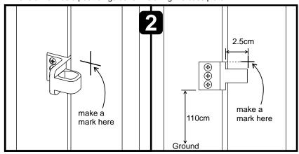
4: install the base plate after aligned to the mark
